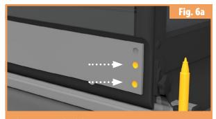
Sydney ENCLOSURE: Using the template, cedure. For SYDNEY enclosures, the MOOVER device is to be placed at least 100 mm from the edge of the module. CAUTION! Mark the two
