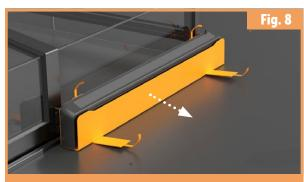
Unfasten the straps with the padding and slide out the attached metallic front cover
