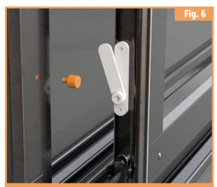
Screw the rubber stop onto the enclosure structure using a C6.3x38 AN9051 screw.
