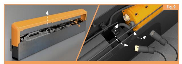
Slide the top cover upwards and disconnect the solar panel (beige) and LED panel (dark grey) connectors from the control unit. CAUTION! — Be sure to pull at the connector, not by the cable Otherwise this may damage the cable. Put the cover and the battery in a safe place to prevent damage during subsequent handling.
