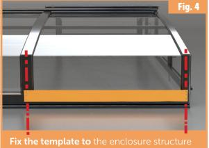
bracket arms. CAUTION! Position the template in such a way that the drilled holes do not interfere with the enclosure running wheel.
