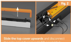
**Slide the top cover upwards** and disconnect the solar panel (beige) and LED panel (dark grey) connectors from the control unit.
